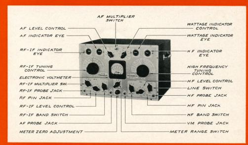
The various controls of the Chanalyst are grouped for greatest ease of operation, as may be seen in the illustration at left, the channel and function of each being clearly designated. The panel is of heavy chromiumplated brass and the calibrations are deeply etched to assure maximum visibility. The electron ray indicators are recessed behind the panel enabling easy observation. The steel cabinet has a dark gray crackle finish and the handles are chromium plated.
