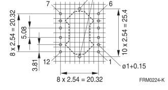
Hole arrangement View in mounting direction (Note half pitch!)
